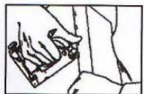
Provided at the rear with a lifting lip for staples
